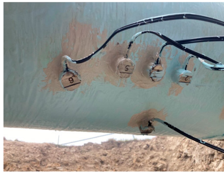
Figure 6: smartPIMS® and matPIMS™ for slurry line monitoring.
