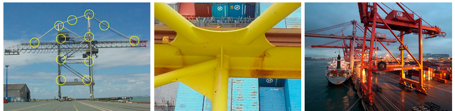
Figure 4: From left to right - Critical welds to be inspected on typical dockside crane, typical weld geometries on crane, dock crane.
