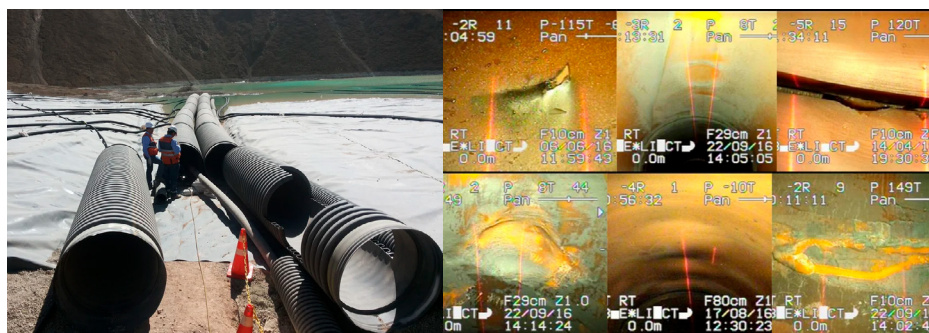
Figure 3: Copper mine pipeline remote visual inspection with VersaTrax.
