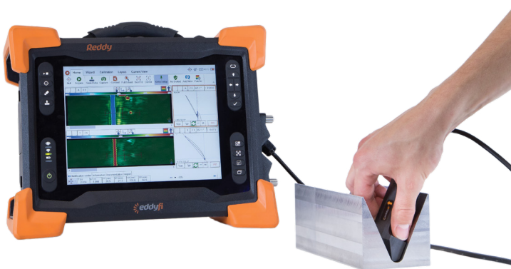
Figure 1: Reddy instrument with ECA gear probes.
