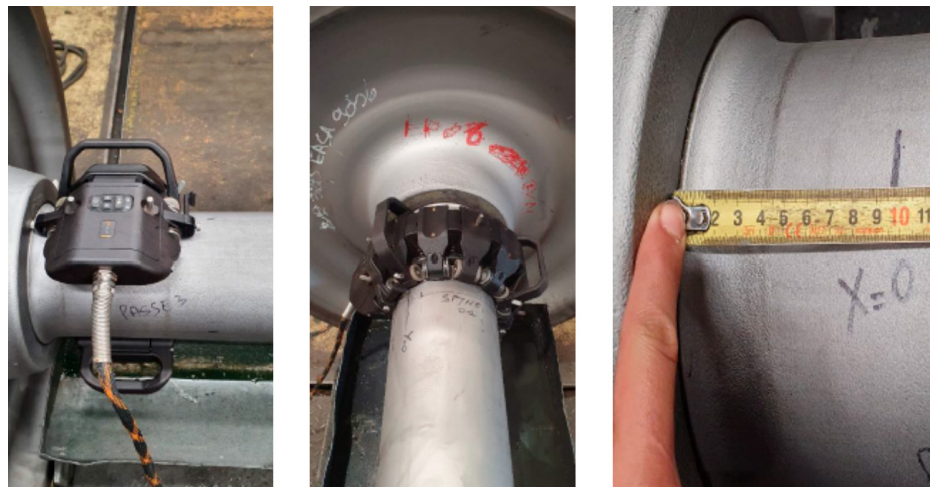
Figure 2: Inspection of the accessible part of the axle body using four successive scans with the Spyne™ probe.
