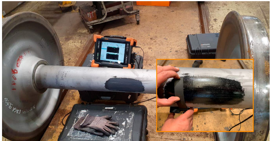
Figure 1: Demonstrating ECA's detection capabilities and sensitivity, an axle body with artificial defects was painted to test inspection efficacy. The flexible ECA probe was used for inspection without altering configuration parameters, showcasing its ability to detect defects through the coating.
