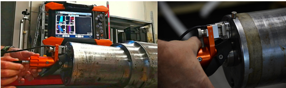
Figure 5: Phased array ultrasonic solution with a unique probe and scanner ensures consistent, reliable results for train axle inspections.
